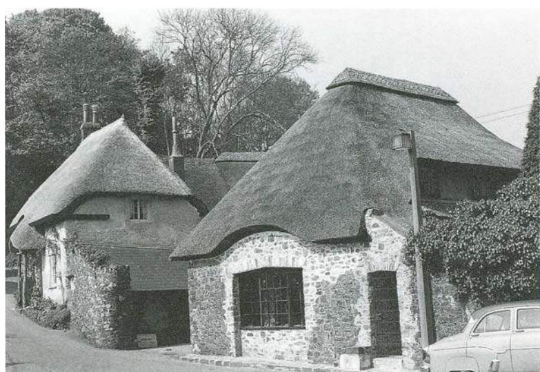
Fig 5 By contrast, the house in Devon (background) roofed in the same material, shows the more rounded outline of a typical hipped roof thatched in combed wheat reed. The house in the foreground is thatched in water reed. (Photograph copyright @ Rural Development Commission)
